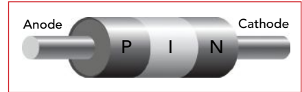
Fig. 5 Typical packaged PIN diode construction.
